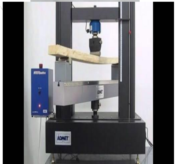
Fig 3.2 Test Specimen & Flexural Testing Machine
