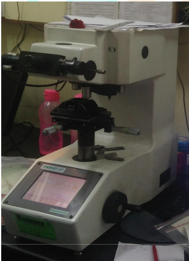
Fig 3.3 Test Specimen & Vickers Hardness Testing Machine.
