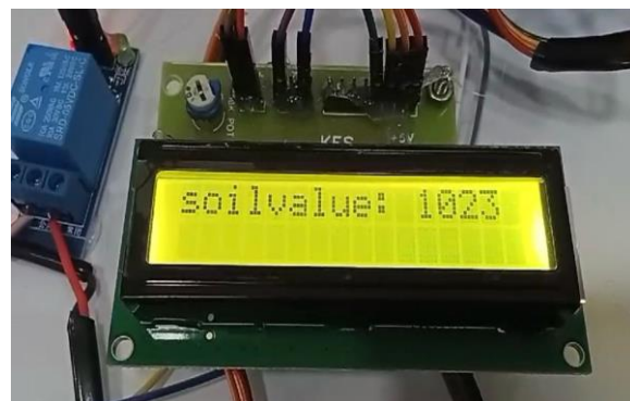
Fig8- LCD Display of Soil Moisture sensor
