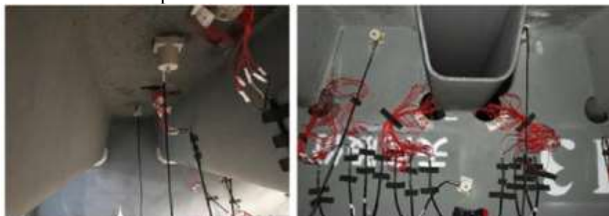
Fig 5.1 phased array ultrasonic testing (source: Chuang Cui 2024)
