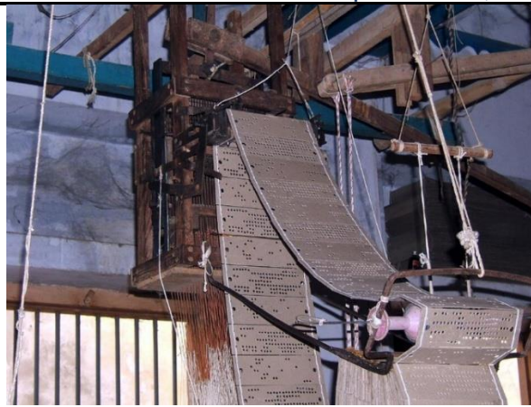
Fig. 5. Punched cards in a jacquard loom
