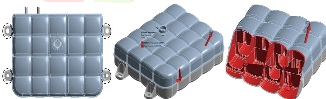
Figure 7. Boundary Conditions and Loading view of Coolant Tank
