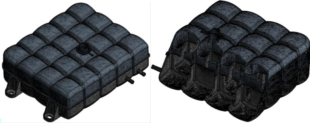
Figure 6. Meshing view of Coolant Tank
